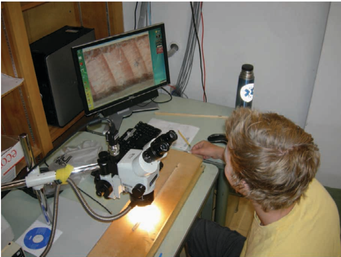
Figure 3. Me using a stage micrometer, a microscope, and the Matlab system to measure intra-annual ring widths.
